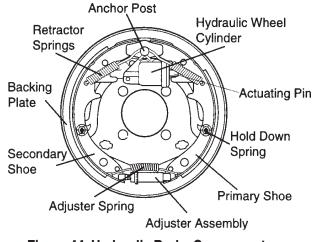
Figure 44. Hydraulic Brake Components
